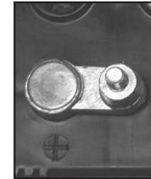
POSITIVE POST HAS LARGER DIAMETER
