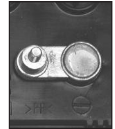
NEGATIVE POST HAS SMALLER DIAMETER
