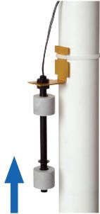
Lift the float up and let go. This will activate the pump. The control unit will run the pump for approximately 25–50 seconds so it can empty all the water in the sump pit. While the pump is active, water will come out of the  $\frac{3}{16}$ " hole that was drilled into the PVC discharge pipe. This is normal. The hole is needed to prevent an air lock within the system. **Do not** obstruct the hole or an air lock may prevent the system from activating.
