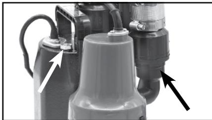
of the main pump, and out of the 3/16" hole in the check valve of the backup pump. This is normal. The holes are needed to prevent an air lock within the system. **DO NOT** obstruct the holes or an air lock may prevent the system from moving water.
