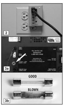
The control unit must receive 115 volts AC +/-5% from the AC outlet. Any voltage lower than 110 volts will activate the "Power failure" alarm. Lower voltages can be caused by utility company brown outs or a heavy power draw from other appliances on the same circuit. Reduce the number of appliances on the circuit.
