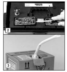
on the right. Place the screwdriver in the middle of the cap on the top of the battery. DO NOT lift the cap by prying it up from the groove on the back of the battery cap. It may damage the vent.
