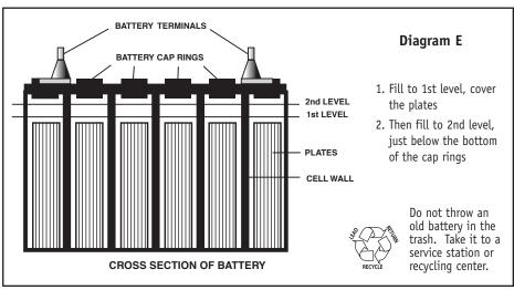
A newly filled battery will sometimes require additional acid after about 20 minutes. Reexamine the fill level, and add additional acid if necessary. The battery acid may bubble at this time and give off a sulfur-like smell, but this is normal. You may top off each cell with a little distilled water, if needed. After the battery has been filled, screw the six (6) caps securely on the top of the battery.
