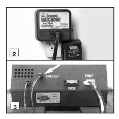
Check the charger plug that fits into the rear panel of the control unit. Make sure it is securely plugged into the control unit.
