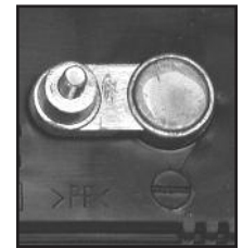
NEGATIVE POST HAS SMALLER DIAMETER
