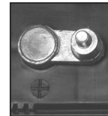
POSITIVE POST HAS LARGER DIAMETER
