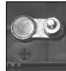
POSITIVE POST HAS LARGER DIAMETER
