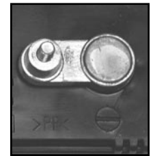
NEGATIVE POST HAS SMALLER DIAMETER
