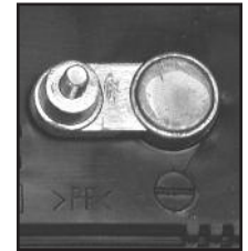
NEGATIVE POST HAS SMALLER DIAMETER
