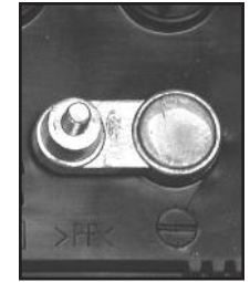
NEGATIVE POST HAS SMALLER DIAMETER
