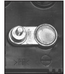
NEGATIVE POST HAS SMALLER DIAMETER
